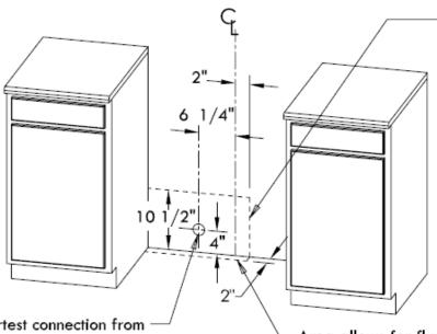
Area allows for flush installation with through-the-wall connection of pipe stub /shut-off valve and rear wall 120V outlet.
