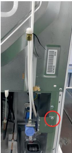
Remove cover machine room on the back side of refrigerator and unscrew.                                   |
