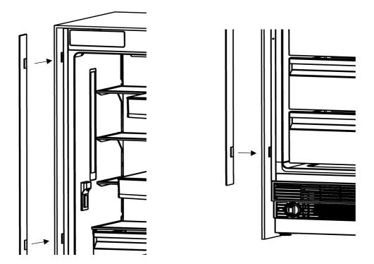
Attach the upper closing part onto the upper connection bracket.
