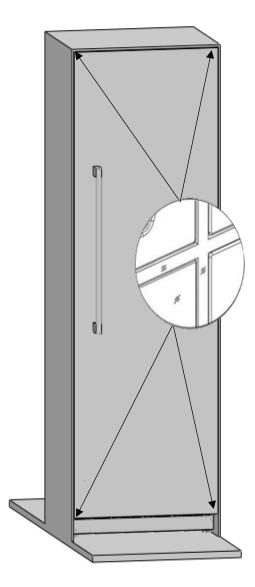
• For products without furniture door, the product is placed using the adjustment part as shown in the figure below.
