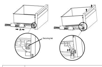
Make sure that the details at the right and left-hand sides are fixed when installing the bin.
