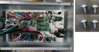
6. The main control board disassembly is completed
