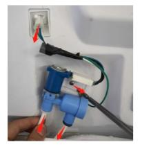
1. Remove the fixing screws and water pipes
