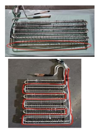
2.Carefully peel the defrost element off of the front of the evaporator.Peel the defrost off the back and remove. Replace in reverse order.
