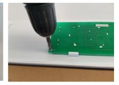
8. Remove the 2 screws securing the display board
