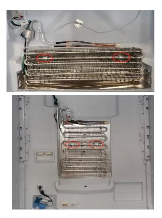
1. Pull out the freezer top drawer. Carefully pull forward on the evaporator to unclip it from the rear wall.Remove the two retaining clips from the front of the evaporator.
