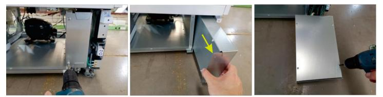
3. Remove the 2 screws that fix the main control board
