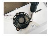
7. Removing the freezing fan
