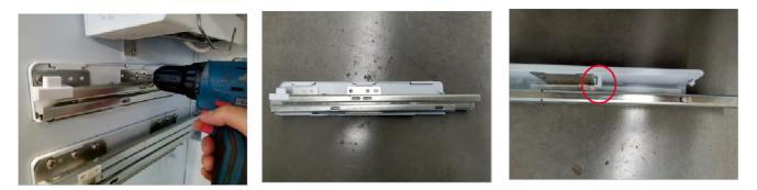
1. Removal of the freezing upper rail fixing screw using a tool 2. Circles are fixed with snaps
