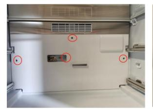
1. Remove the cover plate fixing screws
