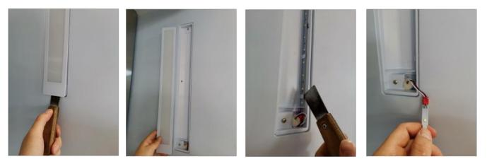
1. Pry open the sidelight cover with a flat shovel 2. Press the light bar snap to remove the sidelight
