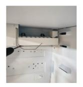
3. Remove the screws holding the ice maker in place
