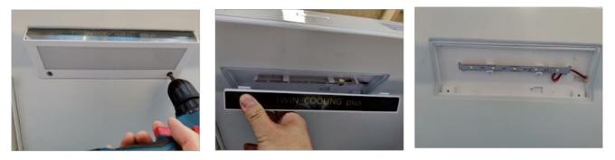
1. Use tools to remove the top light cover screws 2. Press the circle position to remove the top light cover
