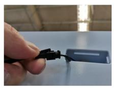
2. Press the connector self-locking catch to remove the magnetic switch
