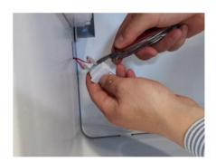
3. Use a screwdriver to pry open the T-terminals
