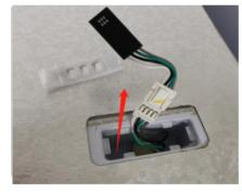
2. Use a screwdriver to pry open the sensor box cover
