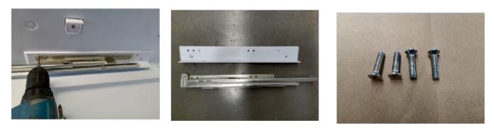
1. Use tools to remove the refrigerated lower rail fixing screws
