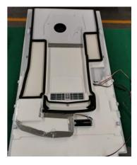
3. Remove the air duct coverplate
