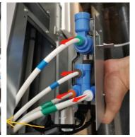
1. Remove the four screws securing the water 2. Pull out the boxand remove valve from the side
