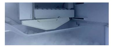
• Install new plastic part: install the upgrade plastic part on the ice maker arm, make sure the ice is not over the ice box.
